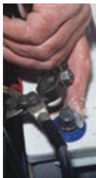
ABOVE: Grease battery terminals and drain watertanks and calorifier
